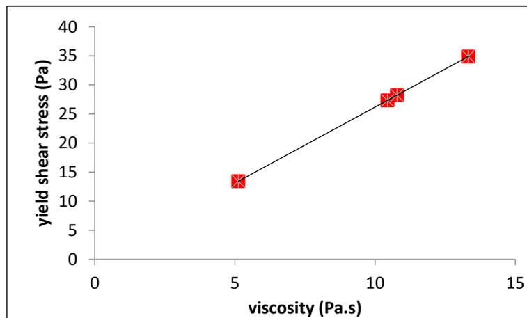
**Fig.5.** Correlation between yield shear stress and viscosity
