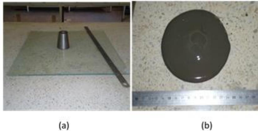
**Fig.2.** (a) Mini slump cone, (b) mini slump spread.
