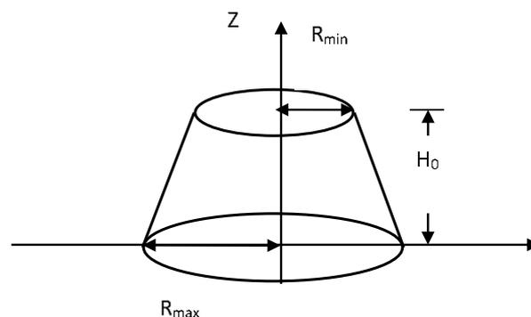
**Fig.1.** Mini slump cone shape.
