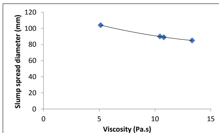
**Fig.3.** Correlation between slump spread diameter and viscosity
