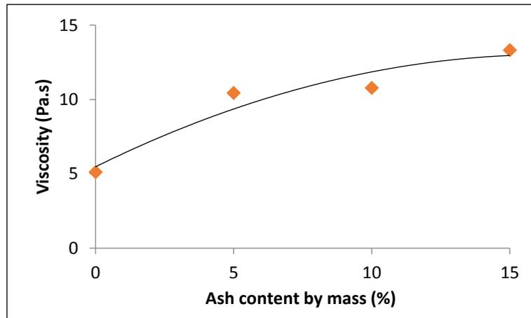
**Fig.4.** Correlation between viscosity and rate of ash content
